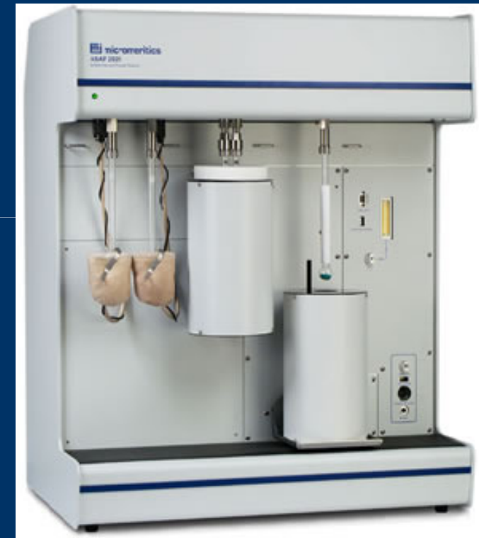
Figure 8. Micromeritics ASAP 2020 device for the specific surface area measurements.
